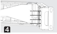
Unfold the rear cable tie bar.
